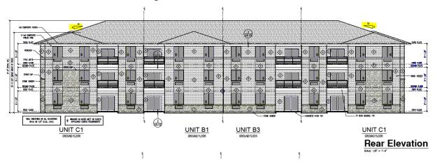
Jason VanAusdall, City Building Official with V&K, noted that 4:12 is a common roof slope for apartment complex buildings. Jason noted that there is no International Building Code justification for why the City of Bondurant regulates minimum roof slope requirements as part of its Zoning Code.
